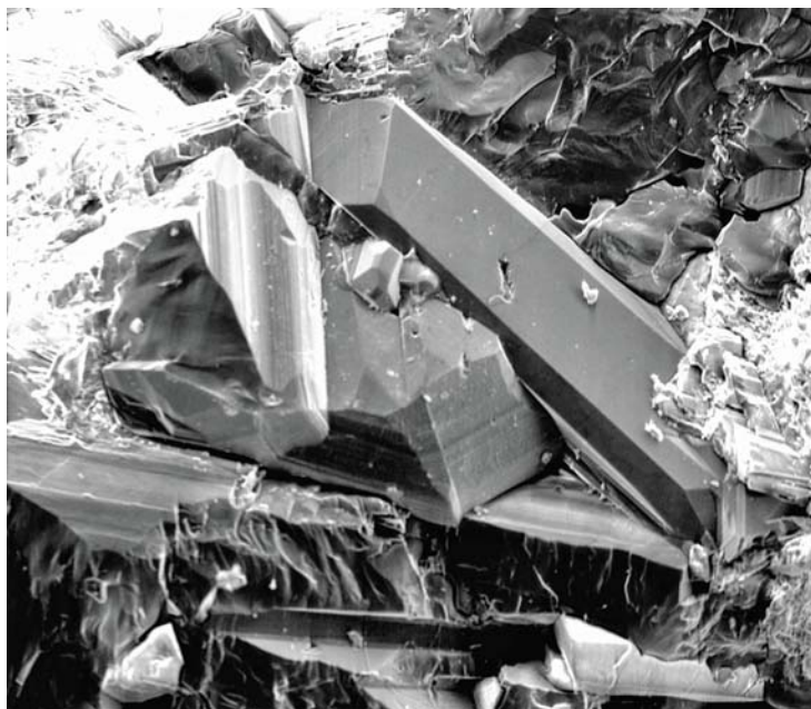
Figure 9. Scanning electron microscope image of allanite-Ce from the lower contact zone at the Silver Hill quarry. Magnification is approximately 260 X. Sample RS-4313.
