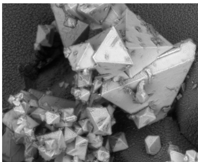
Figure 4. Scanning electron microscope image of magnesioferrite-magnetite series crystals from the Penn/MD Materials quarry, sample RS-4142. Magnification is approximately 740 X.
