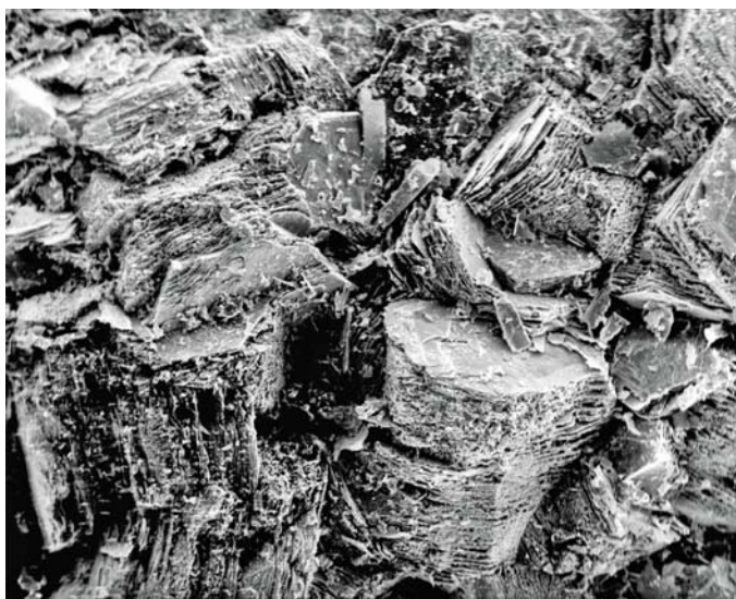
Figure 6. Scanning electron microscope image of pyroaurite from the Penn/MD Materials quarry. Magnification is approximately 76 X. Identification confirmed by SEM-EDS analysis. Sloto collection RS-4218.
