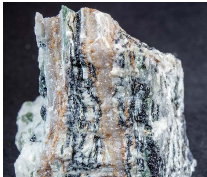
Figure 1. Magnesioferrite-magnetite series in magnesite from the Penn/MD Materials quarry, sample RS-4250.
