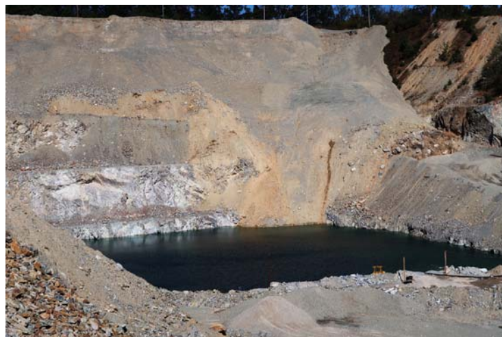
Figure 8. Photograph showing landslide in the Penn/MD Materials quarry (right of center). The flooded fifth level is in foreground. Photograph taken on October 11, 2019.
