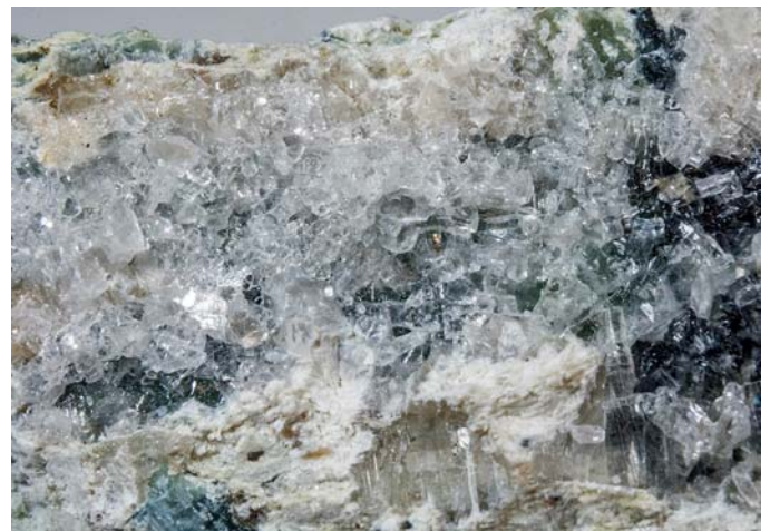
Figure 4. Colorless brucite crystals from the Penn/MD Materials quarry. Field of view is 1.2 cm. Identification confirmed by SEM-EDS analysis. Sloto collection RS-3177.
